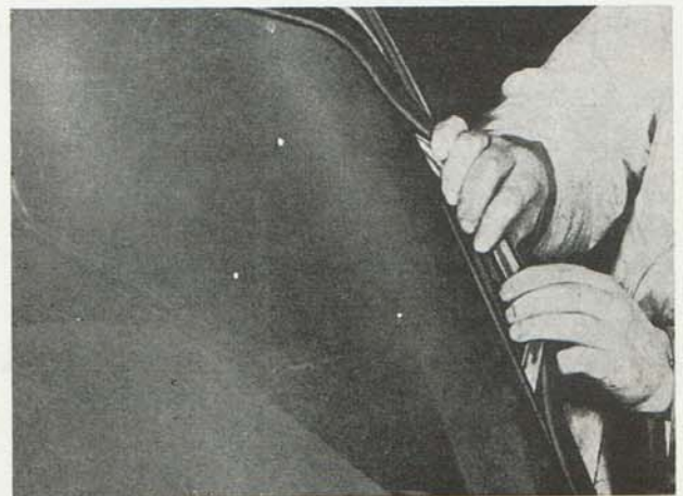
Fig. 58. Removing rubber strip
